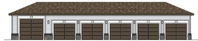
④ FRONT ELEVATION SIX CAR HC GARAGE
